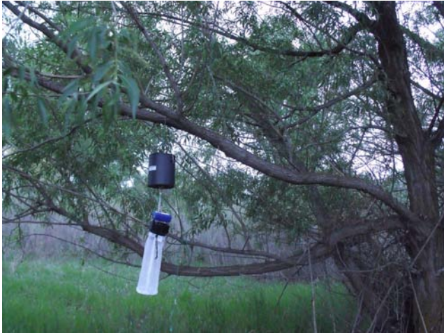
CDC CO 2 Light Baited Traps are deployed at sundown and retrieved in the A.M.
